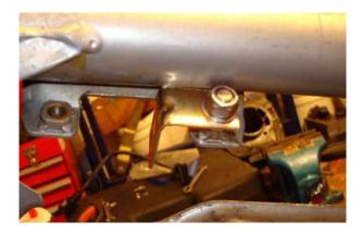
Mount it through the rear coil mount of the frame with a spacer nut or washers between the existing coil mount and the bracket, secure the bracket with a Nyloc Nut.
