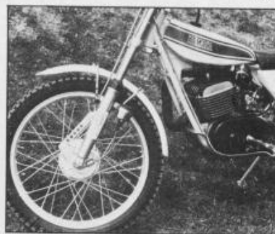
Fork rake is reduced to improve low-speed steering control. Rear suspension has units laid down to give better feel for grip. Dampers are Girling Gas Shocks.
